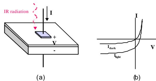
Fig 1 : A photovoltaic IR detector
