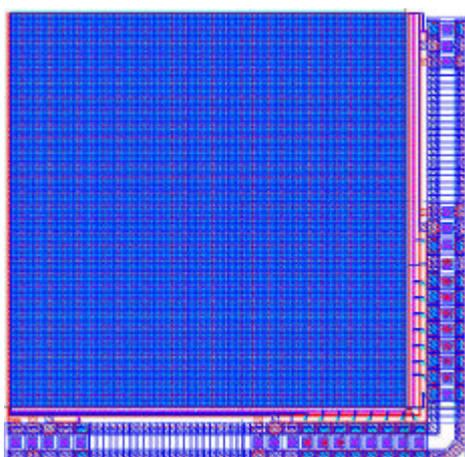
**Fig 13 : The circuit for dark current measurement in 128 x 128 IR FPA**
