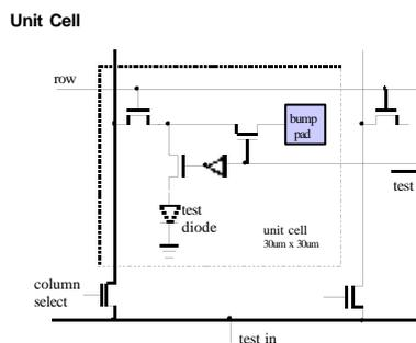
**Fig 11 : The schematic of a unit cell**
