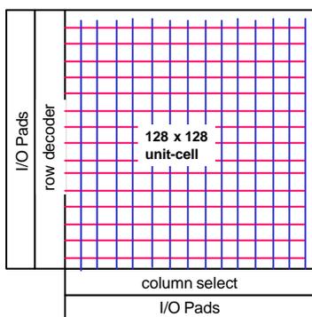
Fig 3 : The architecture of the testing circuit
